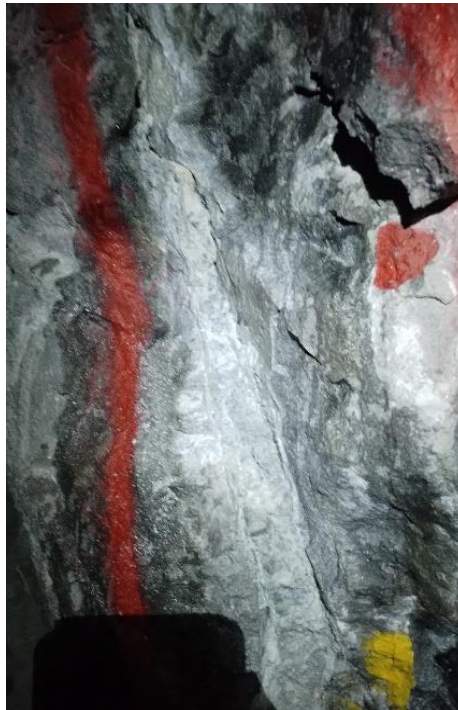
Figure 2a. Photo of URA1 lode located along the northeast wall of the new development decline. The vein at this location is approximately 20 cm wide.
