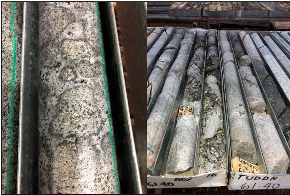
Figure 8-6: Feldspar + silica breccia fill (left) and high-temperature secondary biotite (right)
