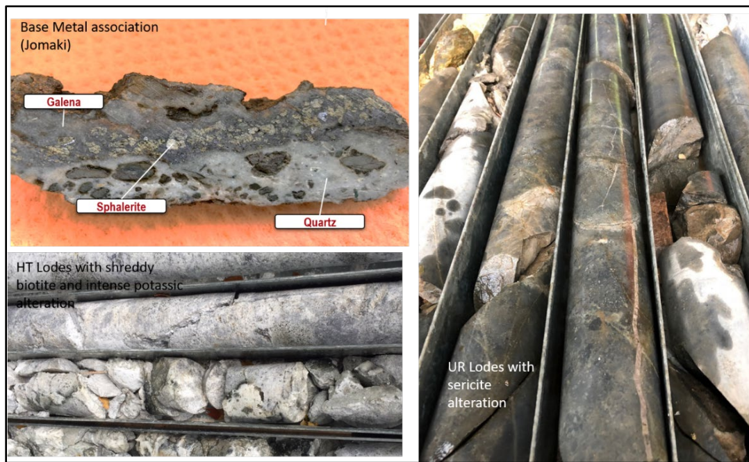
Figure 8-5: Some alteration styles at Tuvatu. Top left image is base-metal and silica dominant; bottom left image is potassium rich minerals, including secondary biotite and potassium feldspar. Right image is typical Upper Ridges style with sericite and carbonate with low-silica.
