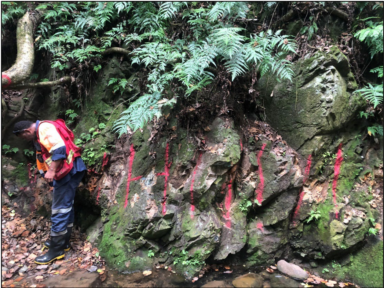
Figure 9-15: Chip channel sampling from a creek exposure (prior to sampling). The red marks represent the sampling intervals.
