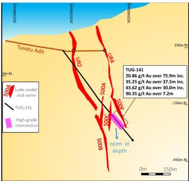
**Figure 1**. Plan view (upper) and vertical section looking E (lower) of the trace of TUG-141 and selected drill holes relative to the 500 Zone lodes modeled to date. TUG-141 was drilled from underground along the Tuvatu exploration decline. The traces of known lodes UR2 and UR4, and modelled lodes of the 500 Zone feeder are shown in red.
