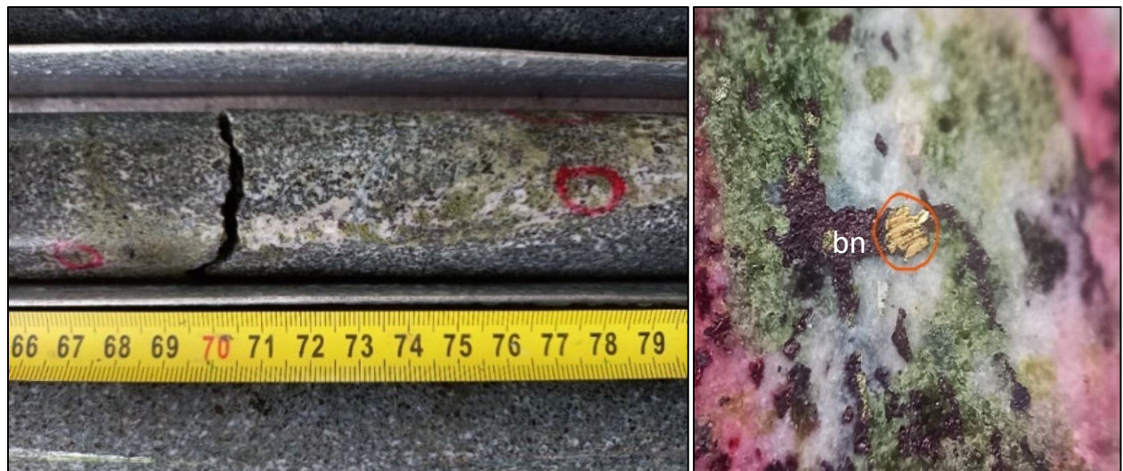
Figure 3: Photographs of the deep intercept from drill hole TUDDH494 at 1106 m depth that returned 12.2 g/t Au and 0.39% Cu hosted in a pervasively altered monzonite exhibiting an assemblage of epidote-actinolite?-orthoclase-biotite-magnetite-bornite and native gold forming an irregular band at low-angle to core axis.
