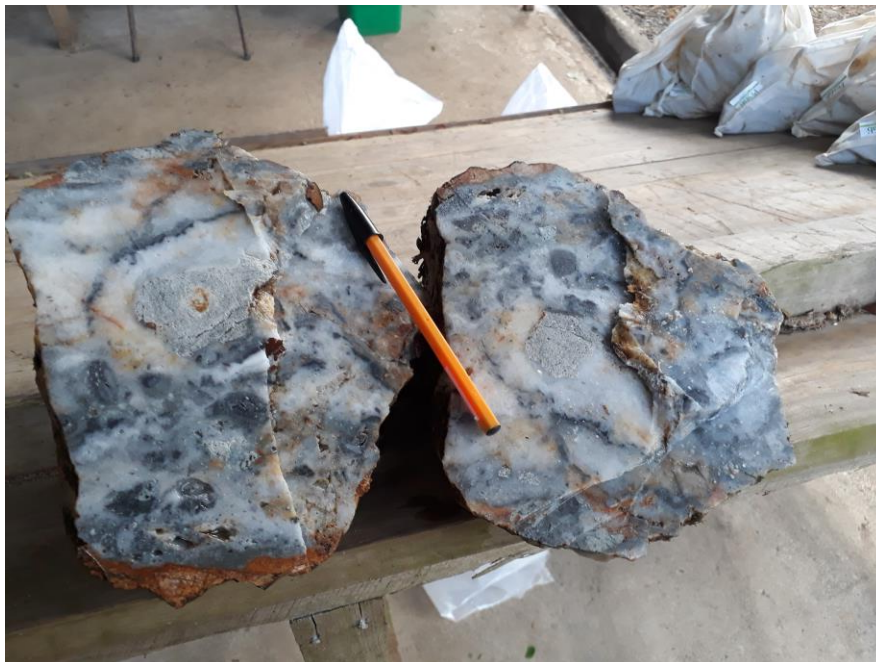
Figure 2: Highly silicified veins in the vicinity of Banana Creek. This exposed Ilesia Vein contains gold and visible galena and sphalerite plus vuggy texture with other sulphides.
