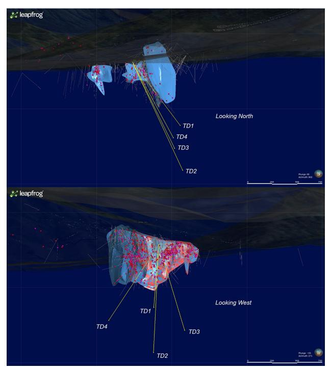
N-S & E-W Section views of proposed drill holes (in yellow), highlighting the existing resource zones (blue) and previous drill holes
